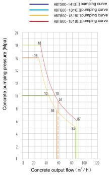
High-pressure pumping Low-pressure pumping
